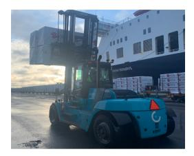
steering cylinder on the chassis and in the tilt cylinders on the mast to minimise maintenance and downtime. One special feature on these lift trucks is a fourth gear that helps lower the rpm with an extra hydraulic pump to maintain lifting speed, a combination that both saves fuel and reduces noise across the long driving distances required in the expansive Karlshamn yard.
