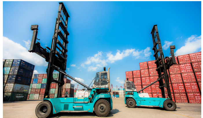
Konecranes empty container handler units working side by side at Haikou Port Container Terminal Co. Ltd, China.
